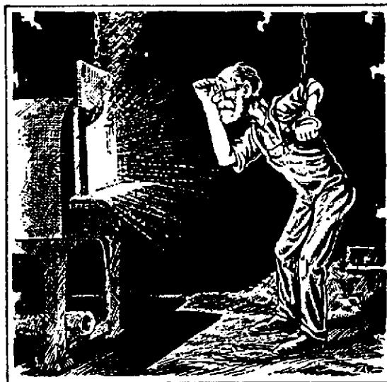
FIG. 1 - THE FIRST OPTICAL PYROMETER.
