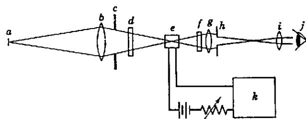
FIG. 6: OPTICAL PATH OF A COMMERCIAL PYROMETER. (A) source, (B) objective lens, (C) objective aperture, (D) absorption filter for temperatures above 1300°C, (E) pyrometer lamp, (F) red filter, (G) microscope objective lens, (H) microscope aperture stop, (I) microscope ocular, (J) eye, (K) instrument for measuring lamp current. (After NBS Monograph 41).
