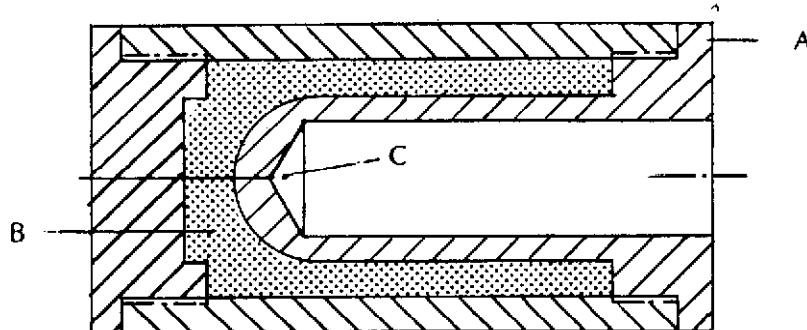
FIG. 2: A PRIMARY BLACKBODY CONFIGURATION: (A) high-density purified graphite, (B) pure metal (C) target upon which the pyrometer is sighted.
