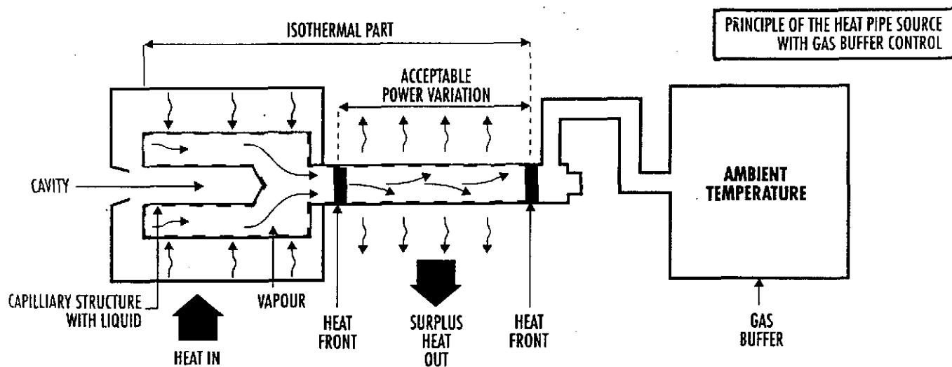
FIG. 5: A SINGLE-TEMPERATURE RADIATING SOURCE WHOSE TEMPERATURE IS CONTROLLED BY A GAS-BUFFERED HEAT PIPE
