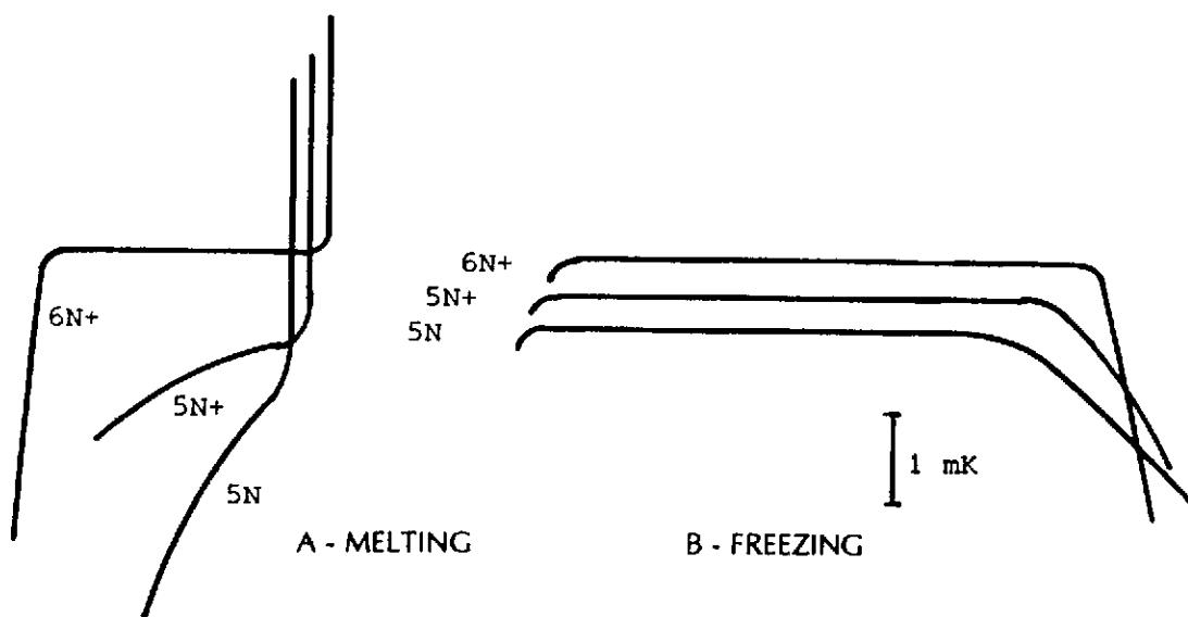
FIG 8: (A) typical melting curves of metals of three purities (B) typical freezing curves
