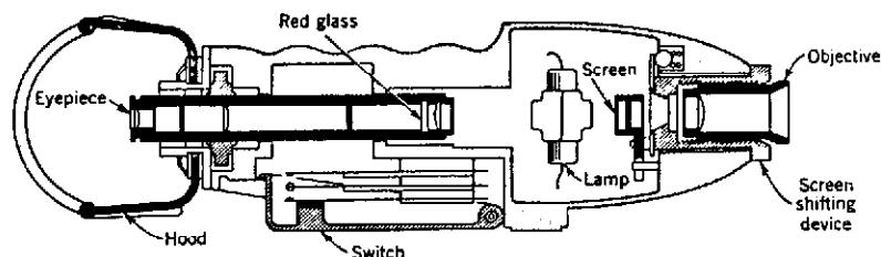
FIG 7: REALIZATION OF A COMMERCIAL PYROMETER: The arrangement of pyrometer elements by Leeds and Northrup. This pyrometer does not include emissivity compensation; most modern pyrometers do.
